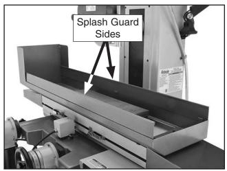
Figure 25. Splash guard sides installed.
